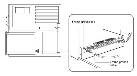
The frame ground cable recommended has a AMP 1-480435-0 housing and 170203-2 or 60711-1 contacts.
